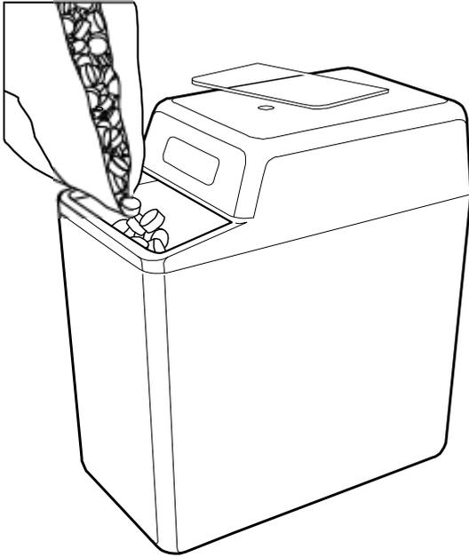
**DO NOT USE FINE OR GRANULAR SALT AS THIS WILL CAUSE A MALFUNCTION.**
