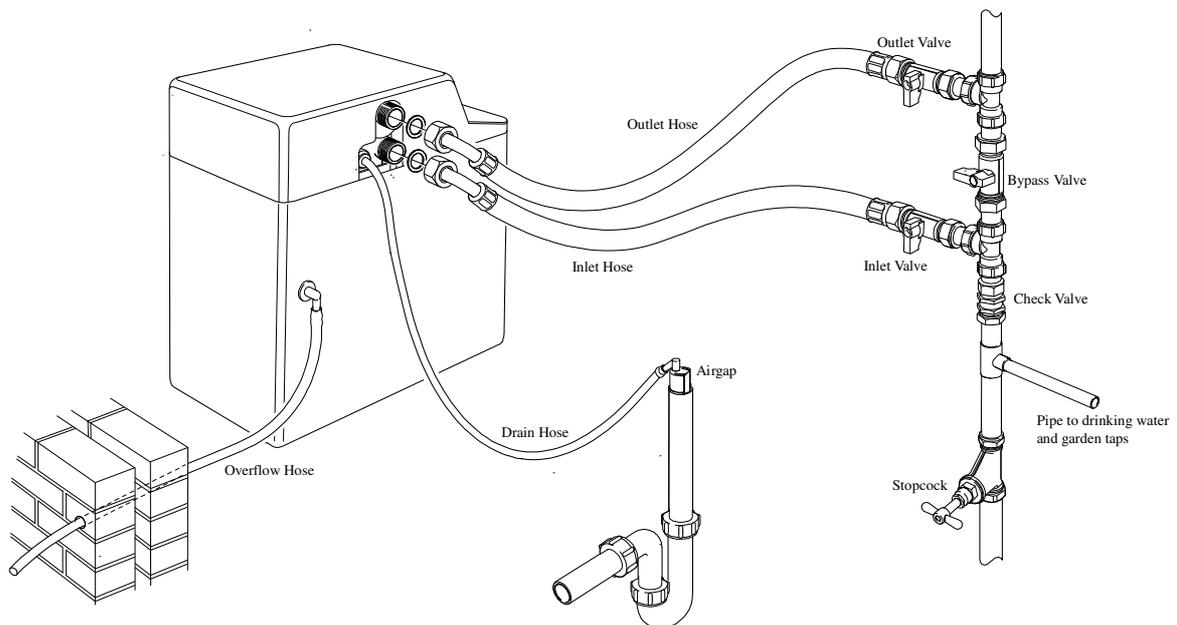
3. Connect a hose between the softener inlet and the inlet valve, then, connect a hose between the softener outlet and the outlet valve.
