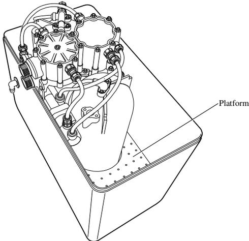
Open the mains stop cock then the inlet, outlet and bypass valves. Open the kitchen sink tap for a few minutes to remove all the air and any colour from the water, and then close the kitchen tap, bypass and outlet valves. Leave for 10 minutes, checking for leaks.
